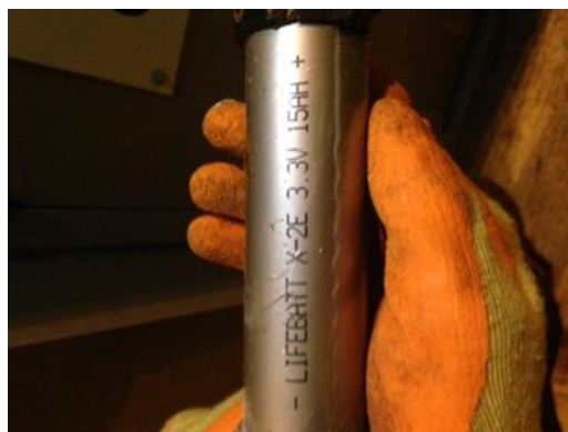
Figure 3: Waste standard LiFePO 4 battery
