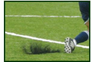
Tire crumb is the most common infill on synthetic turf fields.
