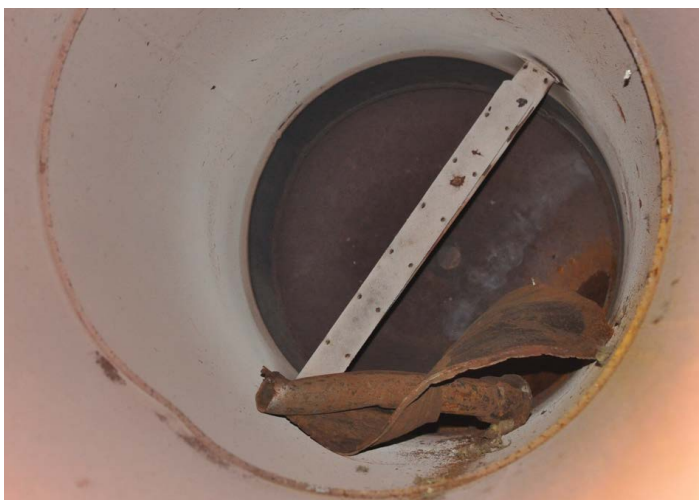
Figure 10. Piece of bottom drain piping and a section of the bottom head
