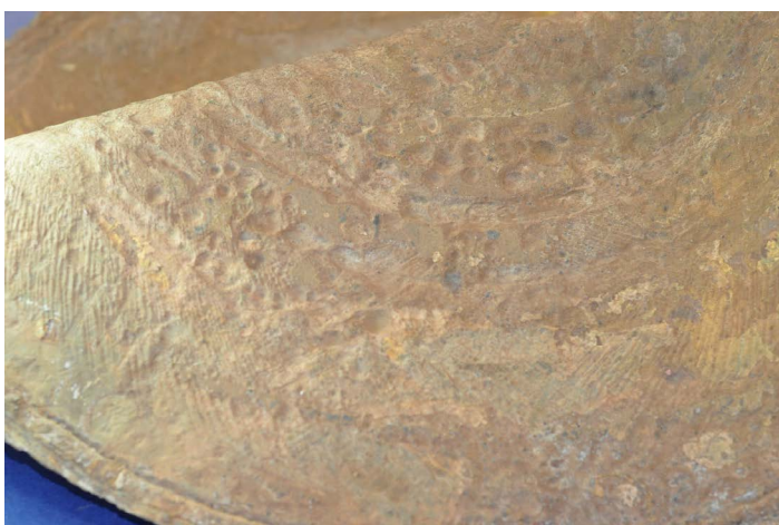
Figure 9. Interior “surface of the moon” condition of the tank circle that separated from the SCR vessel during its catastrophic failure on April 3, 2017. The tank circle was installed in 2012
