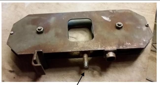
Fig1: CAT Head with hole for retaining pin
